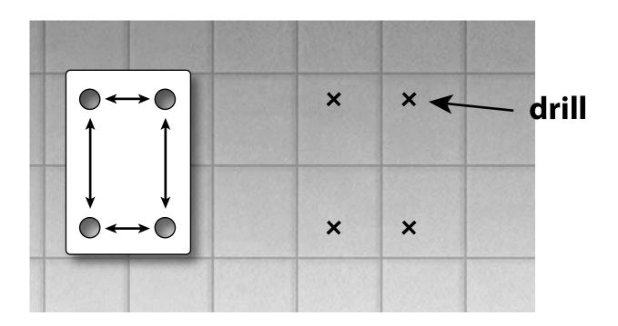
Step 6: Hammer wall plugs in drilled holes, then place the back box over the holes and screw into wall.
